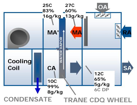
CDQ can produce supply air with <u>dew point lower</u> than the coil chilled water temperature or refrigerant suction temperature
