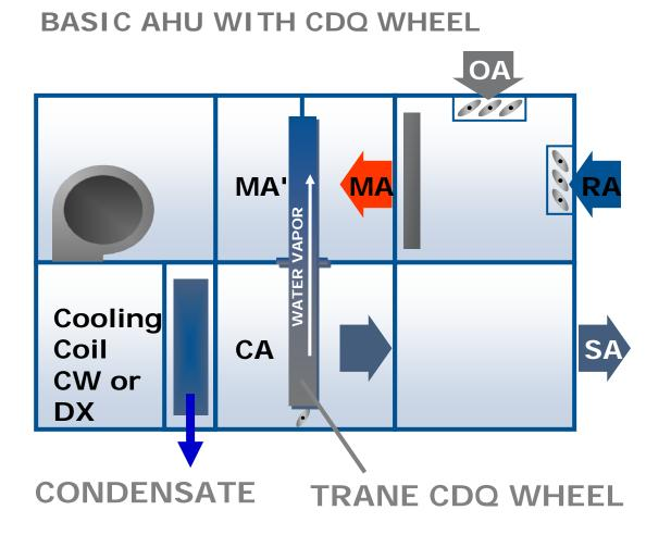
A "Series" <u>Desiccant wheel</u> used to improve the <u>dehumidification</u> ability of a cold coil
